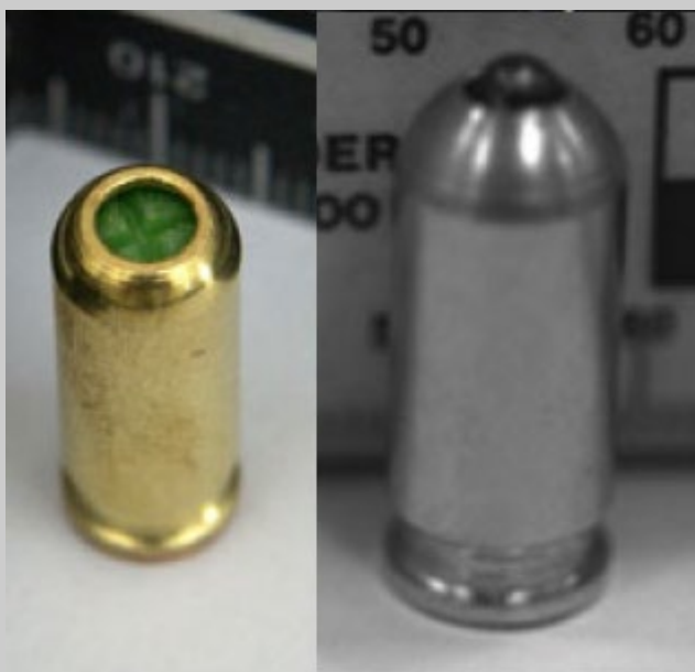
Left: an unmodified blank round; right: a blank round converted through the addition of a metal sphere. 171
