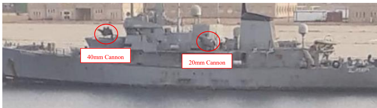
Figure III Image showing retrofitting of weapons to OPV Alkarama (Ras Lanuf – 26 April 2019)
