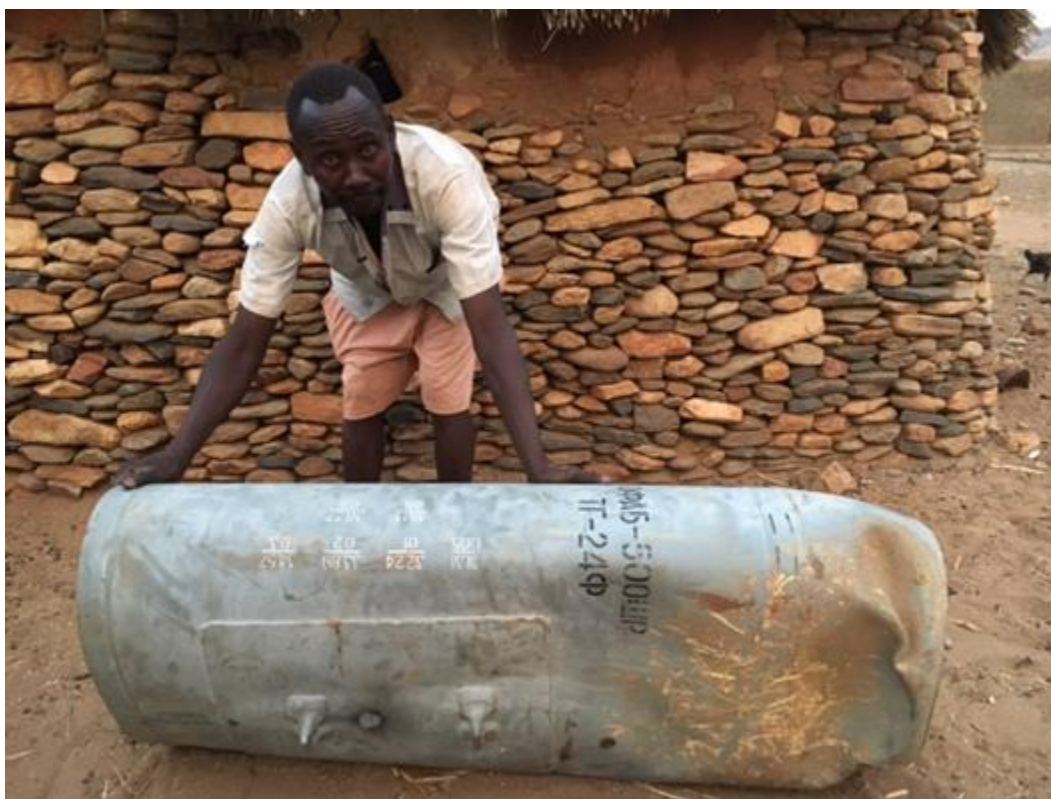
This image shows the forward section of an OFAB-500ShR bomb. This is a large, parachute-retarded, high explosive fragmentation aircraft bomb consistent with SAF's Su-24 attack aircraft. It's a very large bomb carrying over 100kg of explosives and is entirely unguided - a 'dumb' gravity bomb. Its use in a civilian populated area would constitute an indiscriminate attack. The community reported that the bomb killed a 22 year old woman and destroyed an area of civilian houses. The repeated use of unguided bombs and other explosive weapons with wide area effects in the vicinity of densely populated civilian areas would violate the prohibition on indiscriminate attacks. © Transformedia CiC, April 2016
