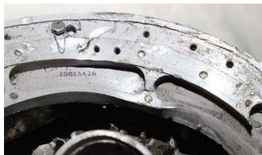
Figure 51.51. Jet engine part of a cruise missile used in the Houthi attack in September 2019 on ARAMCO installations in the KSA. Serial number in the format “100XXXXX” (100 followed by five digits)
