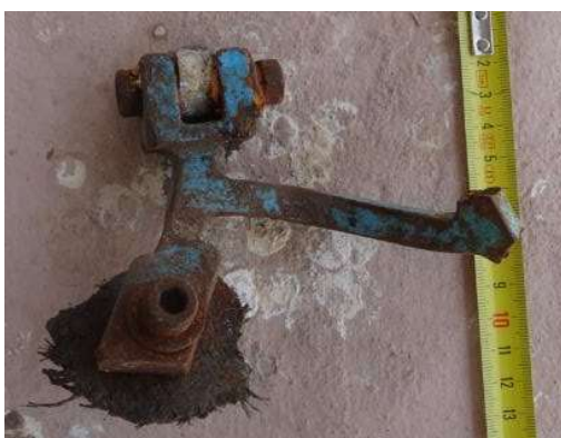
Figure 51.48. Broken jet engine suspension bracket
