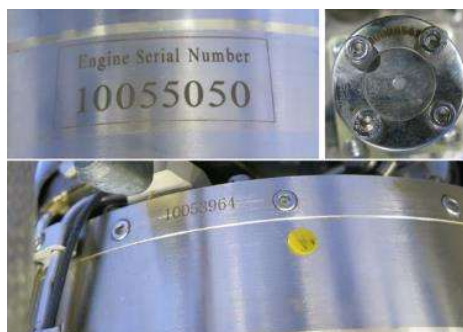
Figure 51.61. Serial number in the format "100XXXXX" (100 followed by five digits) on a jet engine seized by the UK in 2022
